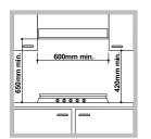
If the hob is installed beneath a wall cabinet, the latter must be situated at a minimum of 700 mm above the hob.
